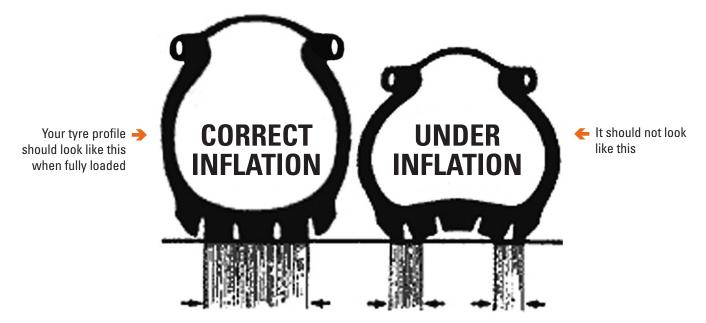
Most of us run tyres that are under inflated. This increases the heat in the tyre and dramatically shortens tyre life, and will cause uneven wear.
